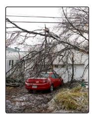
Any downed or fallen wire should be treated as live and dangerous, and you should stay away. Fallen power lines are dangerous because they carry an electric current that can cause serious or even fatal injuries. If you encounter a fallen wire, keep yourself and others away, and call 911 and Southwestern Electric Power Company immediately.
